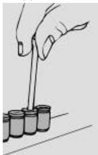
**Figure 5 – Allen wrench to loosen and tighten the air fitting.**
