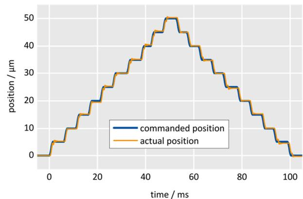
Fig. 9 Stepping motion profile by U-521.24 PLine® stage. Step size: 5  $\mu\text{m}$ , deviation from target position:  $\leq 0.5 \mu\text{m}$ , positioning time:  $< 5 \text{ms}$ . Individual parameter optimization required. Image: PI
