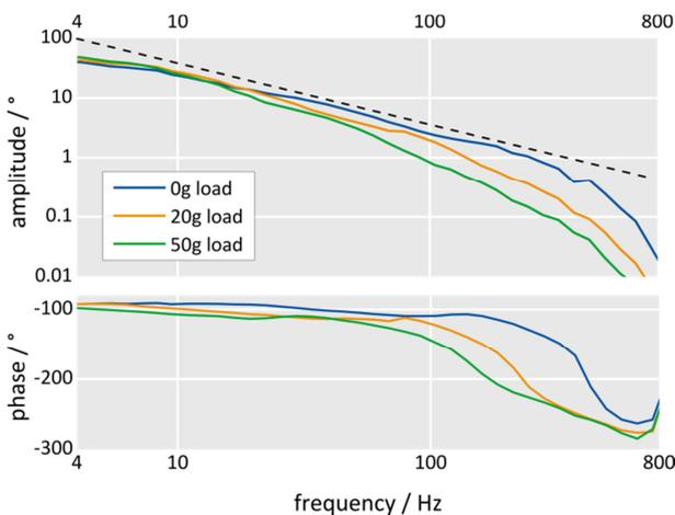
Fig. 21 Open-loop behavior of a PLine® rotary stage displayed in the frequency domain and with different loads. Image: PI
