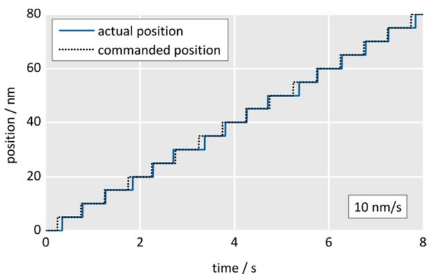
Fig. 14 Trajectory of a customized PLine® stage with a POne sensor, interpolated externally by a PLine® C-867.1U controller. The resolution is lowered to 5 nm, a 20-fold reduction compared to the standard resolution of 100 nm. The commanded position profile is reproduced very precisely. Image: PI
