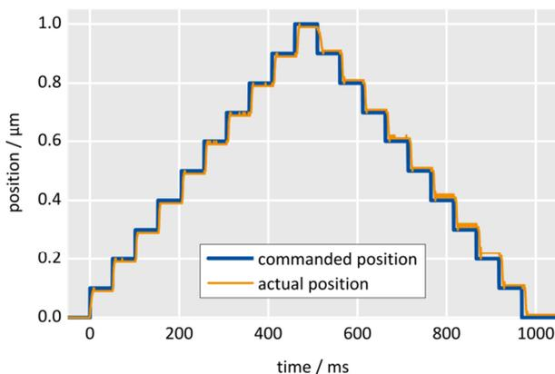
Fig. 11 Stepping motion by a U-521.24 PLine® stage. Step size: 100 nm, settling window: ±20 nm, positioning time: <50 ms. Individual parameter optimization required. *Image: PI*
