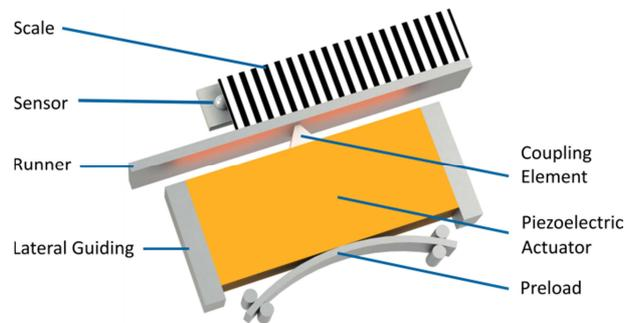
Fig. 1 Schematic diagram of a PLine® motor: The piezoelectric actuator is preloaded against the runner. Electrical excitation of the actuator causes oscillation. This oscillation is converted to forward motion, which is then transmitted to the runner using a coupling element. The position of the runner is recorded by a stationary sensor (encoder), which counts the periods of a grating attached to the runner. Image: PI
