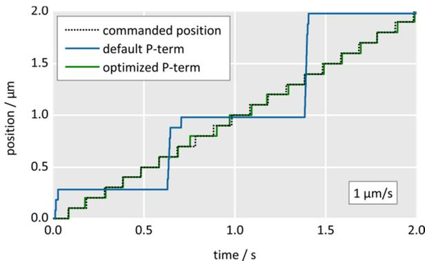
Fig. 13 Ultraslow motion at 1  $\mu\text{m/s}$  before and after P-term optimization. The optimized proportional term causes the stage to closely reproduce the commanded position profile. *Image: PI*
