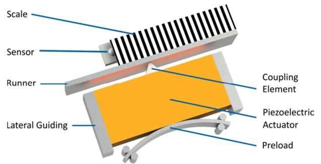
Fig. 1 Schematic diagram of a PLine® motor: The piezoelectric actuator is preloaded against the runner. Electrical excitation of the actuator causes oscillation. This oscillation is converted to forward motion, which is then transmitted to the runner using a coupling element. The position of the runner is recorded by a stationary sensor (encoder), which counts the periods of a grating attached to the runner. Image: PI
