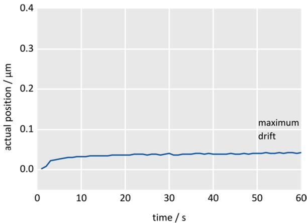
Fig. 20 Position drift of PLine® positioning system with anti-drift modification. Image: PI
