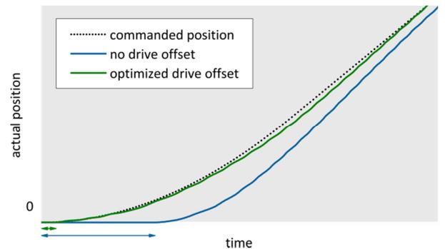
Fig. 5 Adjusting the motor drive offset parameter (0x48) reduces the time delay before starting (indicated by arrows), which is caused by initial stiction between coupling element and runner. Image: PI
