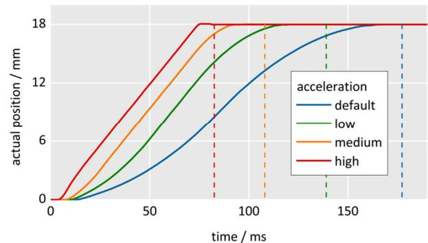
Fig. 4 The positioning time can be reduced using higher closed-loop acceleration (0xB) values. The dashed lines mark the time of settling for an example PLine® linear stage. Image: PI
