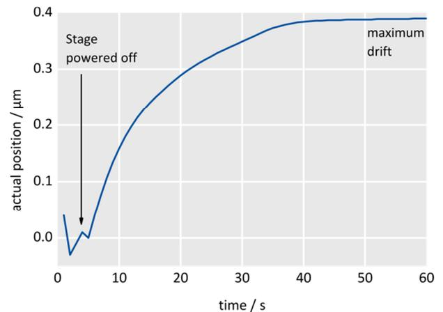
Fig. 19 Position drift example of a typical piezomotor. Image: PI
