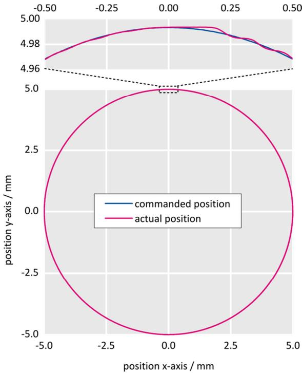
Fig. 17 Moving in a circle using an U-751.24 PLine® XY-stage and a C-867.2U2 controller. The zoom-in shows one of the four reversal points (here y-axis). When the direction is reversed, the maximum following error occurs due to stiction (here approx. 3  $\mu\text{m}$ ). Image: PI
