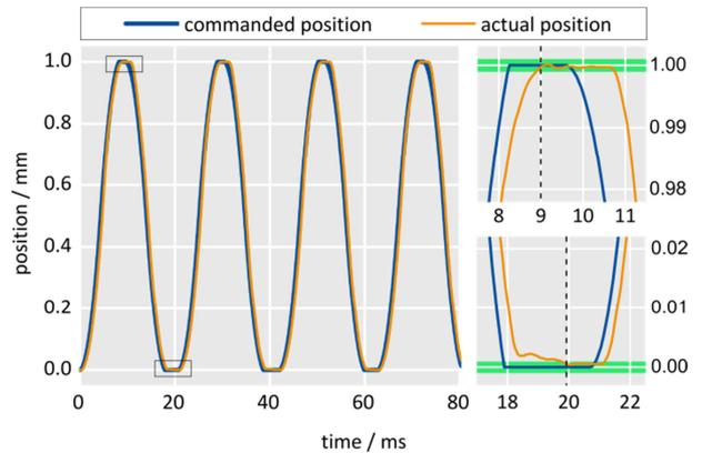
Fig. 10 Scanning application by U-521.24 PLine® stage. Image: PI
