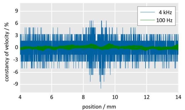
Fig. 12 Constancy of velocity versus position; recorded several times at two different sampling rates. Small local changes in velocity have significantly more impact at high sampling rates. *Image: PI*
