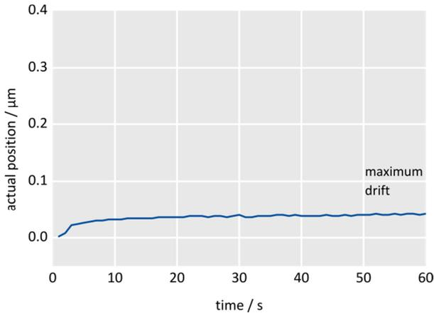
Fig. 20 Position drift of PLine® positioning system with anti-drift modification. Image: PI
