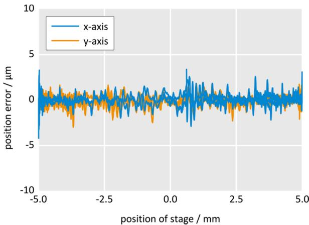
Fig. 18 Following error of both x-axis and y-axis with respect to the position of the stage. Image: PI
