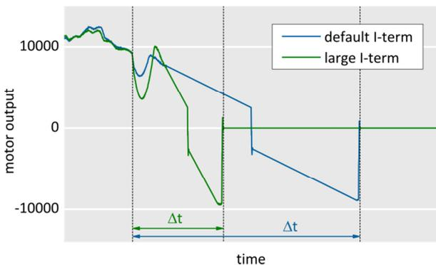
Fig. 7 Increasing the I term of control parameter group 1 reduces the time  $\Delta t$  the controller operates within this control parameter group. At the end of each  $\Delta t$ , the controller switches to settling mode (control parameter group 0). Image: PI
