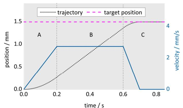
Fig. 2 Example of a position and velocity profile created by a PLine® controller for motion from 0 mm (start) to 1.5 mm (target position). It can be divided into three regions: acceleration (A), constant velocity (B), and deceleration and settling (C). Image: PI
