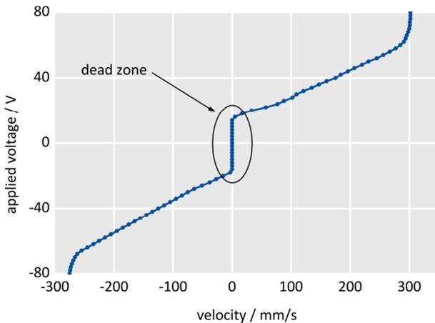
Fig. 16 Typical piezomotor open-loop voltage speed characteristics curve. There is no movement at operating voltages up to the breakaway level which is approximately 16-18 V for this stage. The dead zone is one of the main nonlinearities of piezomotors. Note: A motor output value of 32767 corresponds to the maximum motor output voltage (0x7C; here 80 V). Image: PI
