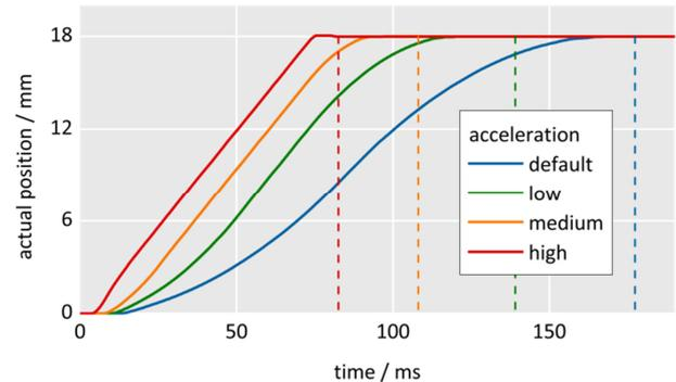
Fig. 4 The positioning time can be reduced using higher closed-loop acceleration (0xB) values. The dashed lines mark the time of settling for an example PILine® linear stage. Image: PI
