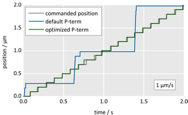
Fig. 13 Ultraslow motion at 1 µm/s before and after P-term optimization. The optimized proportional term causes the stage to closely reproduce the commanded position profile. Image: PI
