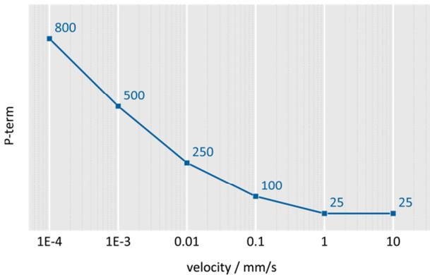
Fig. 15 Exemplary P-term vs. velocity diagram of a PLine® linear stage, plotted on a logarithmic scale. Different values may apply to your stage. Image: PI
