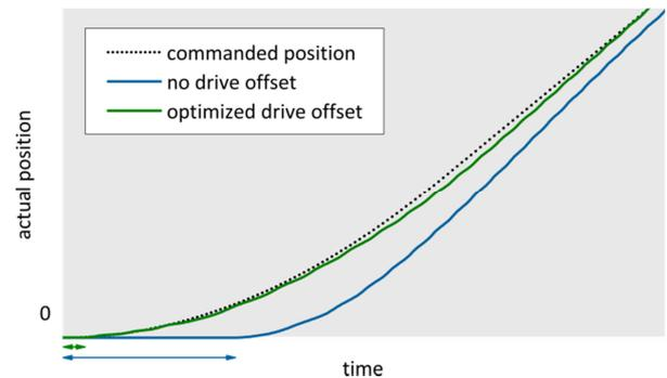
Fig. 5 Adjusting the motor drive offset parameter (0x48) reduces the time delay before starting (indicated by arrows), which is caused by initial stiction between coupling element and runner. Image: PI
