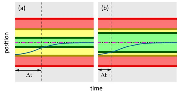
Fig. 8 Zoom-in to the settling region of Fig. 3. Default settling window (a) versus increased settling window (b) leading to earlier settling (for a legend see Fig. 3). Image: PI
