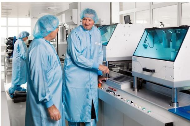
Abb. 3 Workplace for manufacturing PICMA® multilayer actuators in an ISO class 6 cleanroom at PI Ceramic
