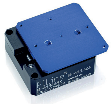
The M-663 PLine® micro positioning stage achieves velocities of up to several 100 mm/s and travel ranges up to several 10 mm. Measuring only 15 mm x 30 mm x 35 mm, the stage can easily be integrated in almost any application
