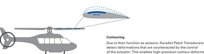
detect deformations that are counteracted by the control of the actuator. This enables high-precision contour deformation in the sub-micrometer range.
