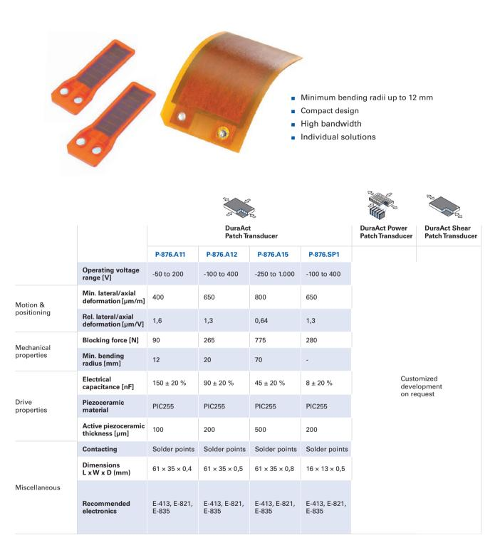
Combined with suitable electronics, DuraAct Patch Transducers are the ideal solution for highly dynamic precise actuators with nanometer accuracy – discover our controllers at www.piceramic.com
