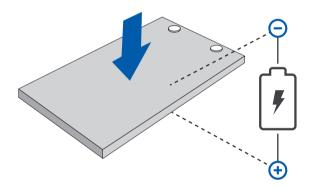
DuraAct Patch Transducers work both as a sensor and as an actuator and can thus dampen undesired vibrations. The phase-shifted sensor signal can also be used as voltage supply for the same piezo element.
