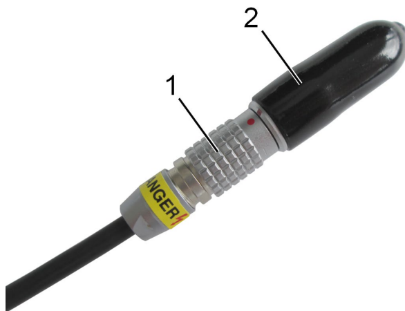
Figure 3: Voltage connection of the P-2x5 with attached shorting plug
