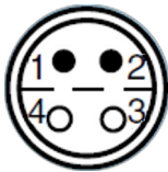
Figure 19: Sensor connector (SGS): LEMO FFA.0S.304.CLAC32Y connector, contact side
