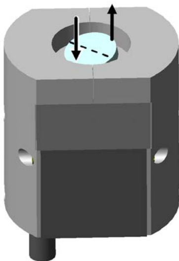
Figure 4: Maximum displacement in the positive direction of motion around axis 2. At the connected channel 2 of the amplifier, the output voltage U_{\text{piezo}} is 100 V. The displacement shown is strongly exaggerated for better understanding.
