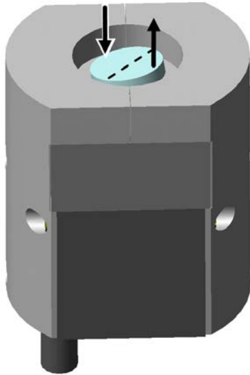
Figure 3: Maximum displacement in the positive direction of motion around axis 1. At the connected channel 1 of the amplifier, the output voltage U_{\text{piezo}} is 100 V. The displacement shown is strongly exaggerated for better understanding.
