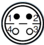
Figure 18: Sensor connection: LEMO connector FFA.0S.304.CLAC32Y, contact side
