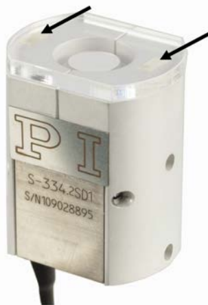
Figure 12: Transport lock of the S-334, the arrows mark the recommended adhesion points
