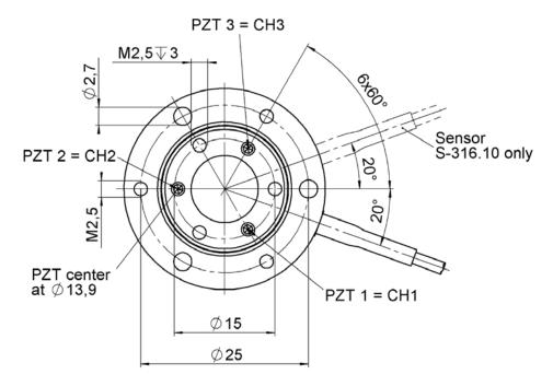
Figure 8: The three M2.5 through holes and the through holes with a Ø of 2.7 mm are to be used to mount the S-31x onto a surface that is connected to a protective earth conductive
