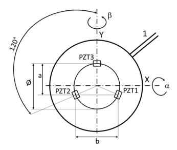
Figure 5: Triple-piezo-drive tip/tilt platform geometry, viewed from above.
