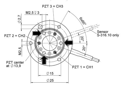
Figure 9: Gray areas mark where glue can be applied onto the S-31x, black arrows mark where to mount a mirror mount
