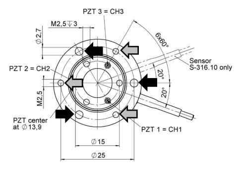
Figure 11: Arrows indicate where to mount the S-31x
