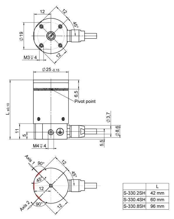
S-330.xSH, dimensions in mm. Note that a comma is used in the drawings instead of a decimal point.
