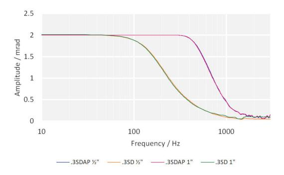
System frequency response with different E-727 controllers and mirror sizes: S-330.2SH
