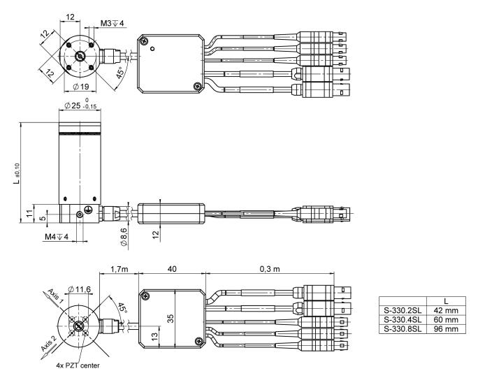
S-330.xSL with cable splitter box; dimensions in mm. Note that a comma is used in the drawings instead of a decimal point.
