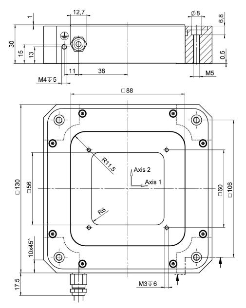
P-734, dimensions in mm. Note that a comma is used in the drawings instead of a decimal point.
