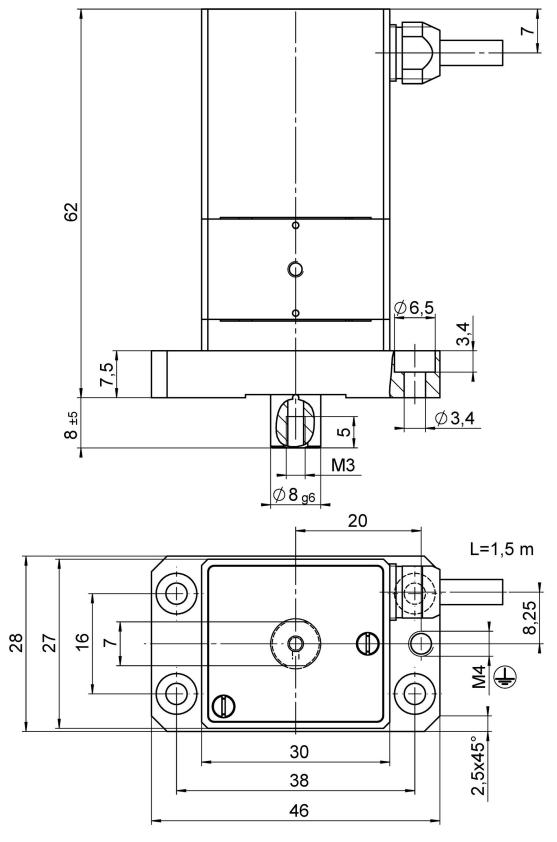
N-111.2A1, dimensions in mm. Note that a comma is used in the drawings instead of a decimal point.
