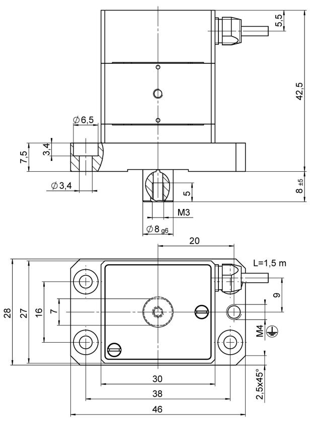
N-111.201, dimensions in mm. Note that a comma is used in the drawings instead of a decimal point.
