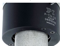
Fig. 7: Objective installed in PIFOC
