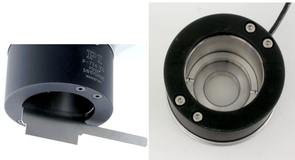
Fig. 11: Objective ring with recesses inside PIFOC can be loosened with key tool
