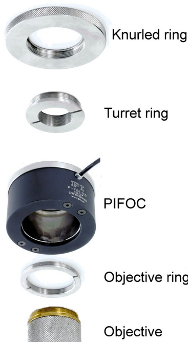
Fig. 3: PIFOC exploded view, as mounted on non-inverted microscope
