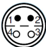
Fig. 18: LEMO connector, 4-pole, for strain gauge sensor (front view)
