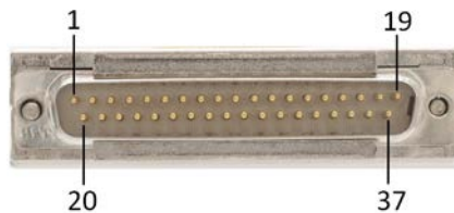
Figure 17: D-sub 37 (m) piezo and sensor connection
