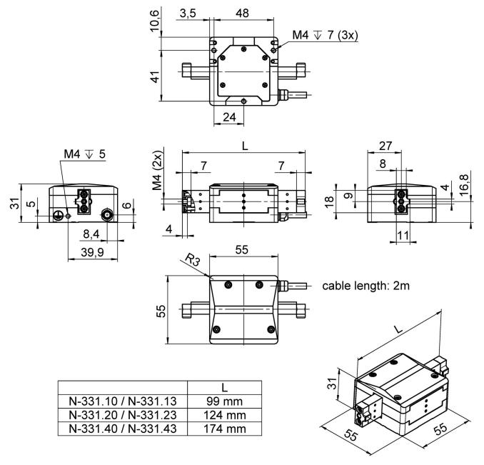
N-331.xx, dimensions in mm. Note that a comma is used in the drawings instead of a decimal point.
