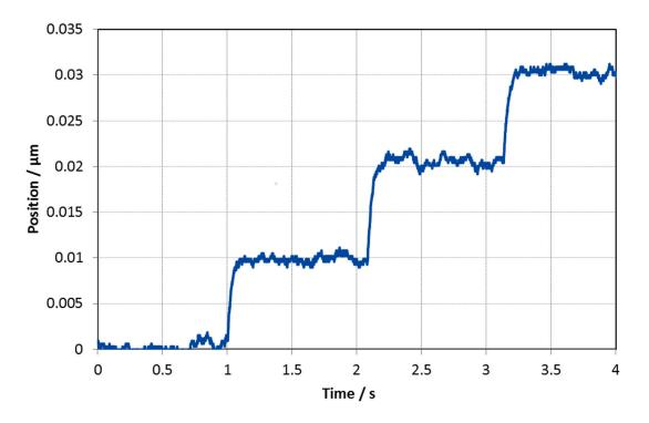
The N-331 drive reliably performs repeatable 10-nm steps. Measured by an interferometer.
