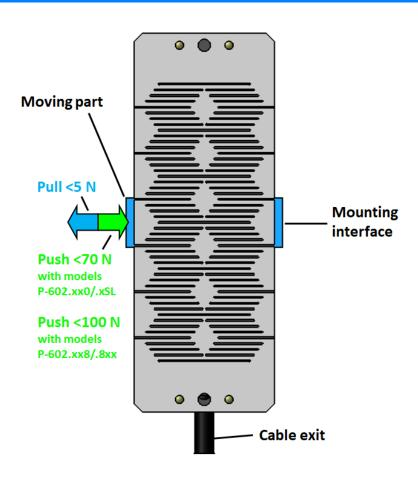
Figure 3: Maximum permissible push and pull forces in motion direction for the P-602
