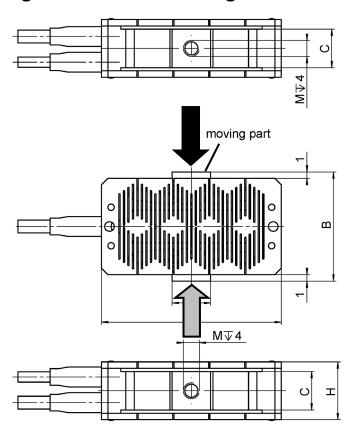
Figure 4: The gray arrow indicates where to mount the P-602 on a surface, the black arrow indicates where to mount a load. Refer to p. 20 for assignment of letters to dimensions.
