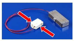
Figure 1: P-602.300 actuator with shorting clamp on the stranded wires, red arrows indicate how to release the stranded wires
