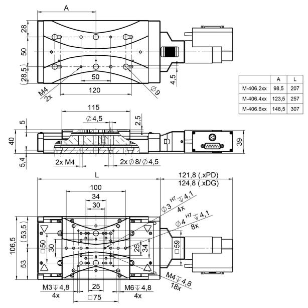
M-406, dimensions in mm. Note that a comma is used in the drawing instead of a decimal point.
