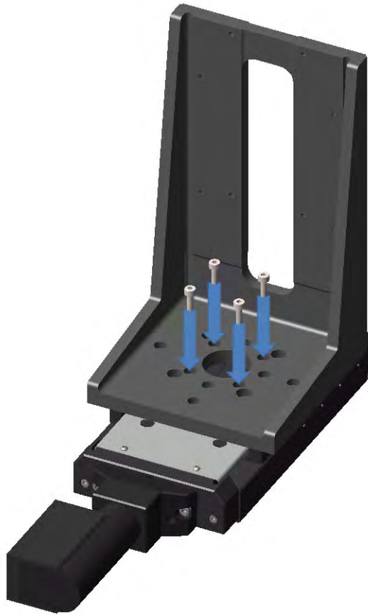
Figure 14: Attaching the adapter bracket to the lower M-406
