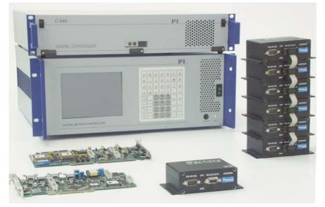
Fig. 4 DC-motor controllers: C-848 and C-880 benchtop/rackmount (background, top to bottom), C-843 PCI bus and C-842 ISA bus cards and Mercury controllers, alone and networked (foreground, left to right)
