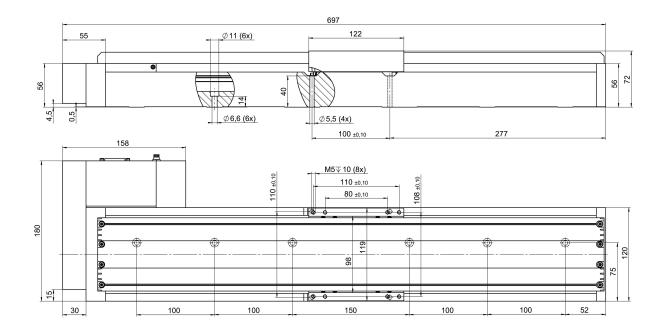
M-417.2PD, dimensions in mm. Note that a comma is used in the drawing instead of a decimal point.
