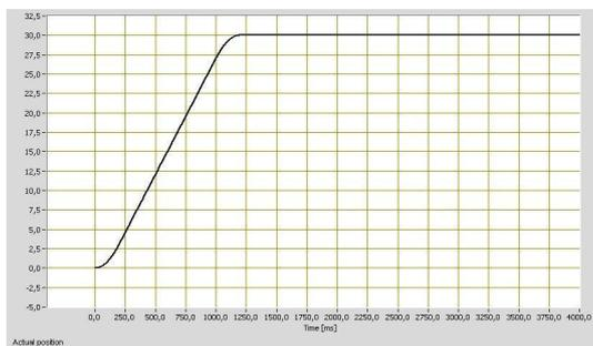
The M-238 requires less than 1.5 seconds for a 30-mm step.
