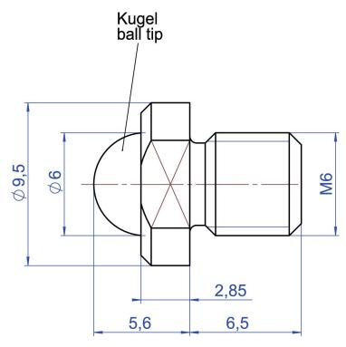
Dimensions of the spherical tip M23550108 (included). Note that a comma is used in the drawing instead of a decimal point.
