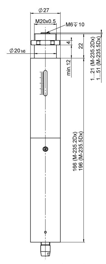
M-235.2DD, M-235.2DG, M-235.5DD, and M-235.5DG, dimensions in mm. Note that a comma is used in the drawing instead of a decimal point.
