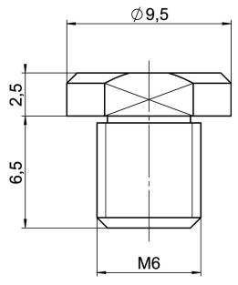
Dimensions of the flat tip M23550107 (included). Note that a comma is used in the drawing instead of a decimal point.
