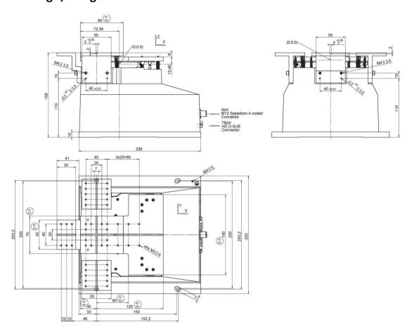
H-206.F2, dimensions in mm. Note that a comma is used in the drawings instead of a decimal point.
