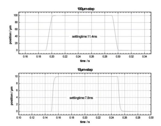
Step response of the P-733.ZCD. Settling time is 10 ms.
