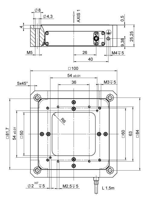
P-733.Z, dimensions in mm. Note that a comma is used in the drawings instead of a decimal point.
