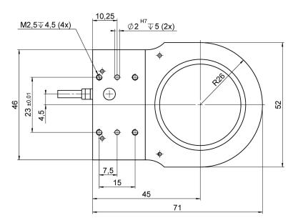
P-725.CDD, dimensions in mm. Note that a comma is used in the drawings instead of a decimal point.
