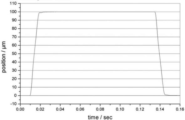
With active control, the settling time is less than 10 ms over the entire travel range.
