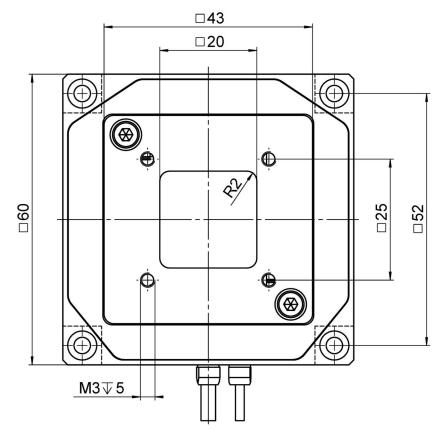
P-612.ZSL, dimensions in mm. Note that a comma is used in the drawings instead of a decimal point.
