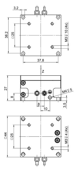
P-611.ZS, dimensions in mm. Note that a comma is used in the drawings instead of a decimal point.
