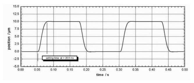
The P-611.ZS needs a settling time of 26 ms for a 10- $\!\mu m$  step with a load of 30 g.
