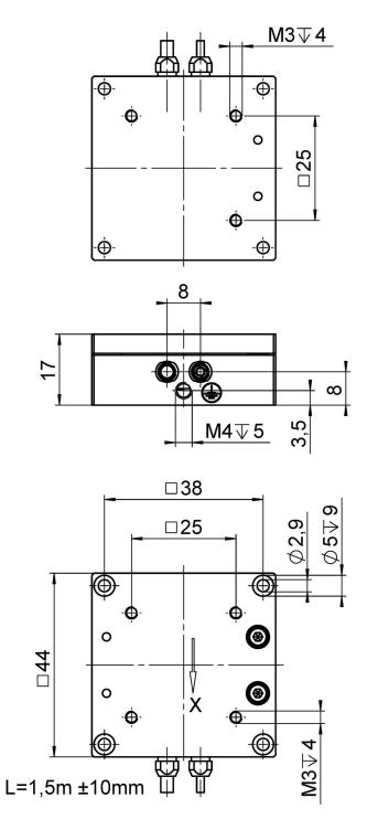
P-611.1S, dimensions in mm. Note that a comma is used in the drawings instead of a decimal point.
