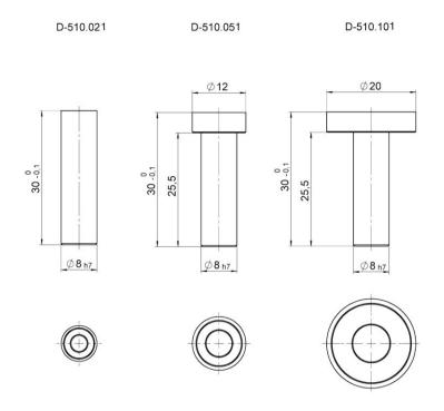
D-510.021, D-510.051 and D-510.101, dimensions in mm. Connector: LEMO FFC00.650.CLA.543, triaxial
