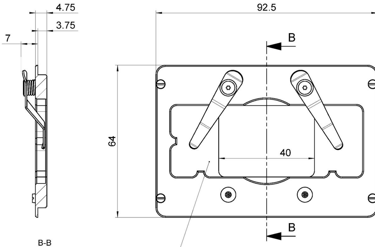
Opening for Standard Microscope Slide
