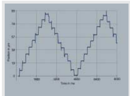
PILine® Piezo linear motor stage performing 1 µm steps. Piezomotors are self-locking. After a stable position is reached, there is no servo dither as common with other linear motors.
