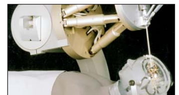
Custom Hexapod designed for neurosurgery Photo: IPA
