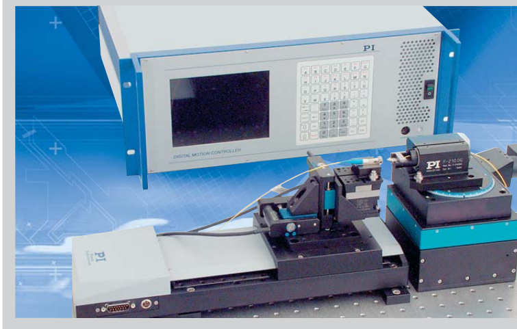
Fiber alignment configuration example. Top: C-880.00D equipped with F-206.iRU IR-photometer card, 2 x C-842.40 servo-motor control cards and E-760.3S0 piezo controller card. Bottom left: M-511.DD precision translation stage with 0.1 µm linear encoder for rapid loading/unloading; F-131.3SD hybrid fiber alignment system with 15 mm travel range in XYZ and 1 nm resolution. Bottom right: M-501.1PD precision vertical stage with 0.008 µm encoder resolution; M-061.PD rotation stage and the discontinued F-210 fiber rotator.
