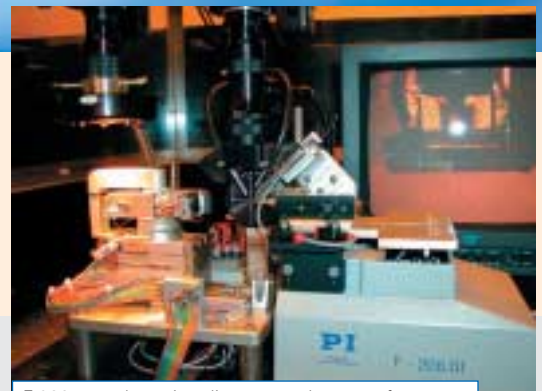
F-206 as a photonic alignment subsystem for automated assembly of fiber pigtailed devices. Courtesy of Aries Innovations, Inc.
