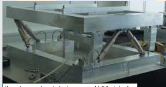
Beyond microsystems technology: custom M-850 robot with a positioning frame measuring some 1.0 x 1.5 meters.
